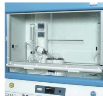
Compact rotary evaporator, which can be neatly installed in a fume hood. The vertical condenser does not take up much space
